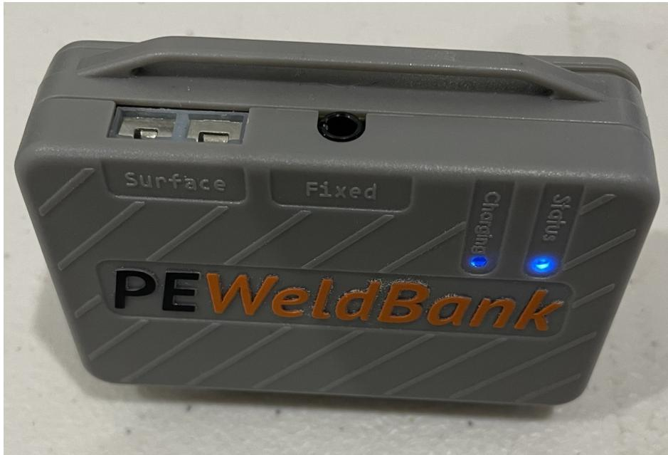
The Sensors dated March 2022 and later allow for connection to the Butt welding machines heater plate internal PT100 probe (where available)
