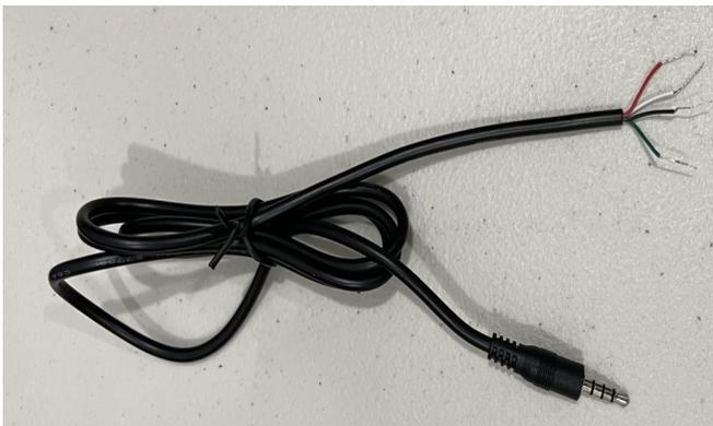
This 1m long lead is included. One end is to plug into the Fixed sensor port (3.5mm 4 pole) the other end has 4 wires allowing fitment of you own plug to suit your machine. (Red = FORCE —, White = RTD —, Green = RTD +, Black = FORCE +. For connection to 2 wire probe join [Red+White] & [Green+Black]
